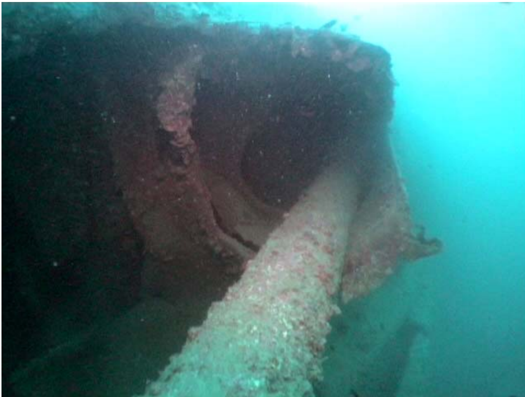
X4/2 - Looking forward along outer Port shaft to where stern tube gland 'should' be.
