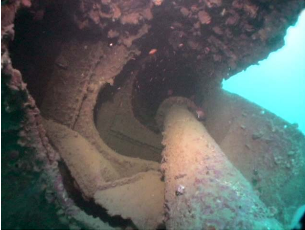
F1 - Distorted web frames and the flange that joins the two 'outermost' lengths of shaft.
