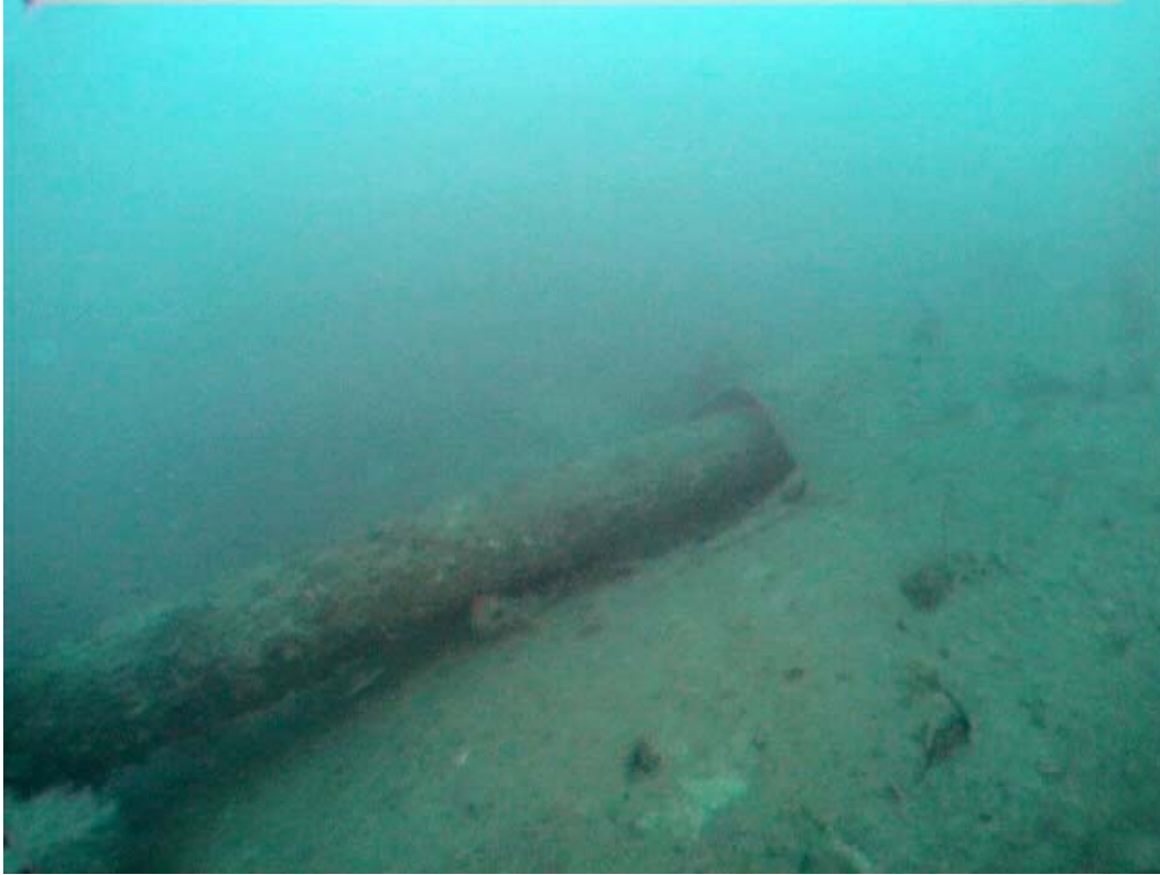
X1- The Starboard outer propeller shaft where it exits the hull from the stern tube gland.
