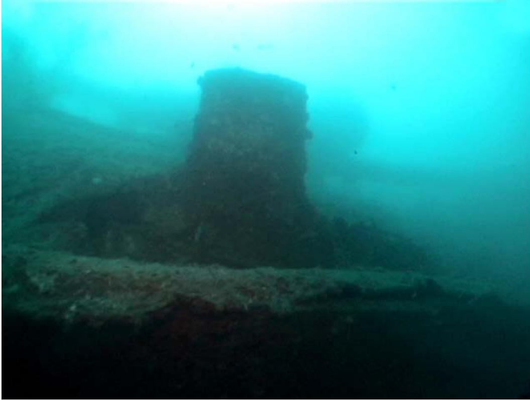
A1 - Only a short stub remains of the outer strut of the outer Starboard A-Bracket.
