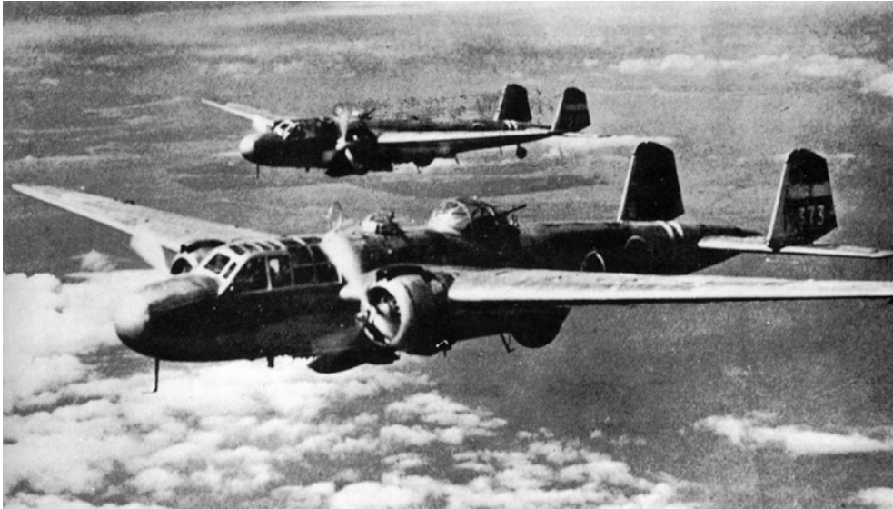
Mitsubishi G3M Type 96 Rikko : Allied code name 'Nell', carried either bombs or torpedoes in the attack (i.e. some carried bombs and some carried torpedoes).
