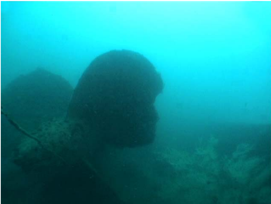
B4- Outer Stbd propeller left. Note disfigured blade. Keel Plate is dark area at right.
